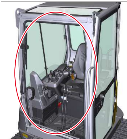
Fig. 101: Opening/closing the entire front window
