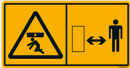
Fig. 18: Crushing hazard lifted load
