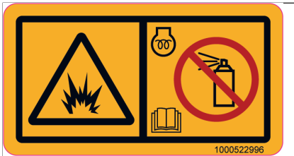
Fig. 31: Air intake (jump start)
