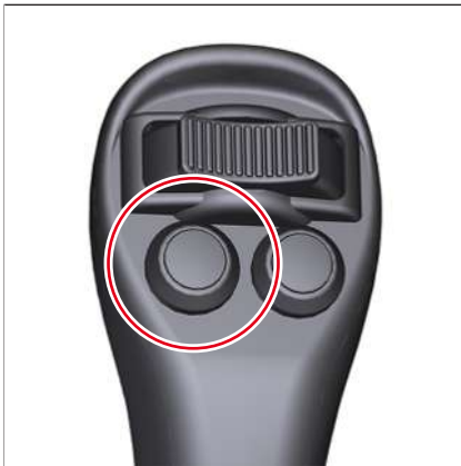
Fig. 194: Switch over AUX II/AUX III
