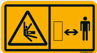
Fig. 19: Crushing hazard in the danger zone
