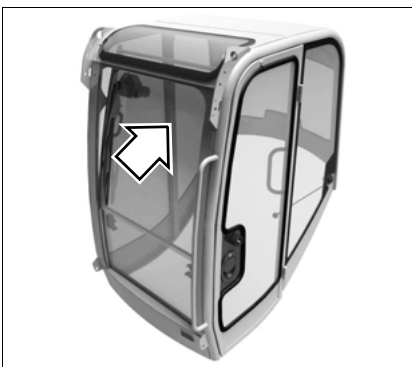
Fig. 97 Opening the front window to a gap
